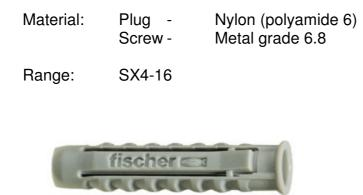
The fischer SX plug has a four-way expansion section compared to conventional two-way expansion plugs. This unique four-way expansion gives a greater load capacity, as the surface area in contact with the substrate is much greater than with standard plugs. Therefore, the SX plug is designed for both solid and hollow building materials.
