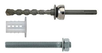
The PBB undercut anchor system is designed specifically for aircrete with FISV resin and threaded rod. The special PBB drill produces a conical hole, which when filled with resin, produces a mechanical interlock which guarantees maximum load bearing capacity with stress free installation.
