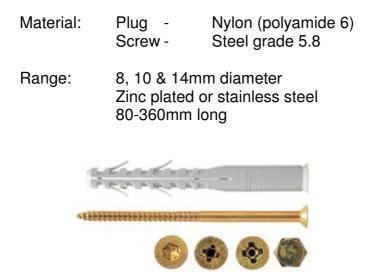
The S-H-R frame fixing operates in the more common two-way expansion, but due to the longer expansion section a deeper embedment depth is used, increasing the load bearing capability in hollow and softer substrates.
