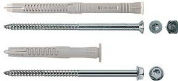
The fischer FUR sets a new standard for the frame fixing. Its innovative expansion section results in the FUR being suitable for virtually all construction materials with high loads and optimum reliability. Anchorage in solid materials is by friction locking. The close-set teeth provide ideal expansion of the fixing in solid substrates, ensuring constant expansion force along the entire anchorage length. The close set teeth expand and form lock in hollow materials.
