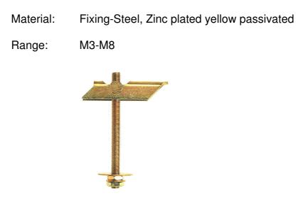
The fischer KD Toggle is the versatile cavity fixing. This fixing can be used in most substrate providing it has a cavity. It ranges from M3 to M8 and comes in varying lengths. It is made from mild steel grade 5.8 and is zinc pasivate. The installation procedure is simple and produces very high loads. Smaller versions of the KD toggle come with spring loaded toggle fixing and a selection of threaded attachments from hooks to eyelets.
