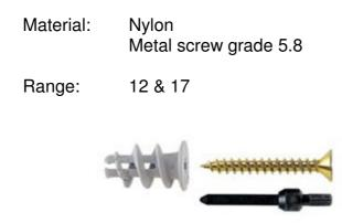
The fischer GKS has a self-cutting thread for rapid installation, there are no pre drilled holes required just a screwdriver or power driver. When installed the anchor is flush with the substrate surface and very little space is required behind substrate. This fixing is for fast installation and is capable of producing fairly high loads.
