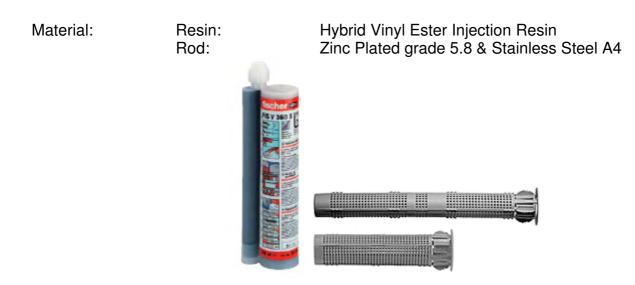
The fischer Injection System FIS V contains a styrene free, quick setting, high quality hybrid resin mortar, which is characterized by its universal suitability for many applications. It achieves maximum strength values in almost all building materials and anchors safely without expansion pressure. The 2 components are mixed together inside the static mixer. A simple exchange of the static mixer allows the cartridges to be reused after they have been opened.
