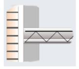
The Omnia system has been developed to provide the direct equivalent of an insitu slab and provides the facility to combine pre-cast and in-situ concrete, offering major benefits to specifiers, engineers and contractors.
