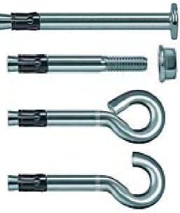
Nail anchor for fast and simple hammerset installation. The anchor expands automatically under load, pulls the cone into the expansion clip and expands against the hole wall.
