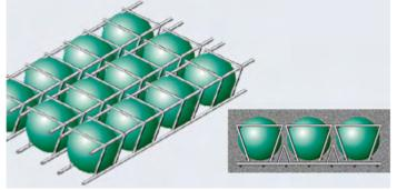
The reduced weight allows the quantity and dimensions of vertical bearing elements, such as columns, to be reduced. Reduced dead weight means a smaller deflection of the slab and also provides scope for savings in foundation design, including fewer piles and/or reduced length of piles.
