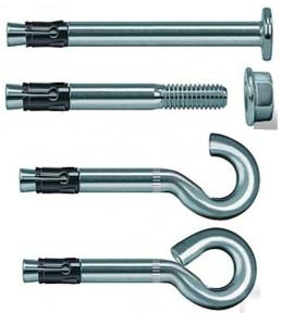
fischer FNA II Nail Anchor for fast and simple hammerset installation. The anchor expands automatically under load, it pulls the cone in to the expansion clip and expands against the hole.
