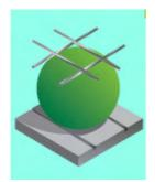
BubbleDeck is a revolutionary method of virtually eliminating concrete from the middle of a floor slab where concrete does not perform any structural function, thereby dramatically reducing structural dead weight. BubbleDeck is based on a new patented technique – the direct way of linking air and steel. Void formers in the middle of a flat slab eliminates 35% of a slabs self weight removing constraints of high dead loads and short spans.
