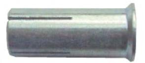
The FDA-R is similar to the conventional Drop In anchor. Its rimmed collar on the fixing ensures the anchor remains flush with the surface at all times even if the hole is drilled slightly deeper then required. To ensure correct installation a setting tool should be used with this anchor. The setting tool required is the EAW H Plus.
